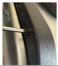
Using the L-Shape TP30 Torx Wrench on the outward-facing OEM screw and pressing your finger firmly on the OEM inward-facing screw unscrew and remove the OEM outward-facing screw.
